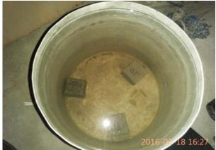
Figure- 2:Specimen submersion in fresh water
