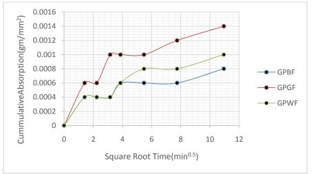
Figure-6: Graphical representation of cumalitive sorption with time function of different samples
