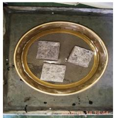
Figure-3: Specimen subjected to unidirectional sorption
